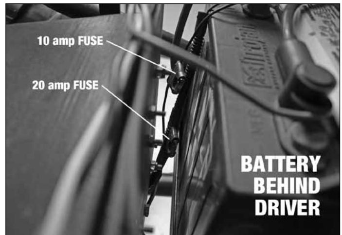
figure 4.25 (10 amp & 20 amp fuses)
